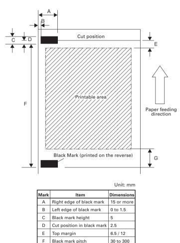
Top margin will be changed by the setting of the memory SW4-8. In the case of 0 (OFF), the top margin is 6.5mm. In the case of 1 (ON), the top margin is 12mm.
